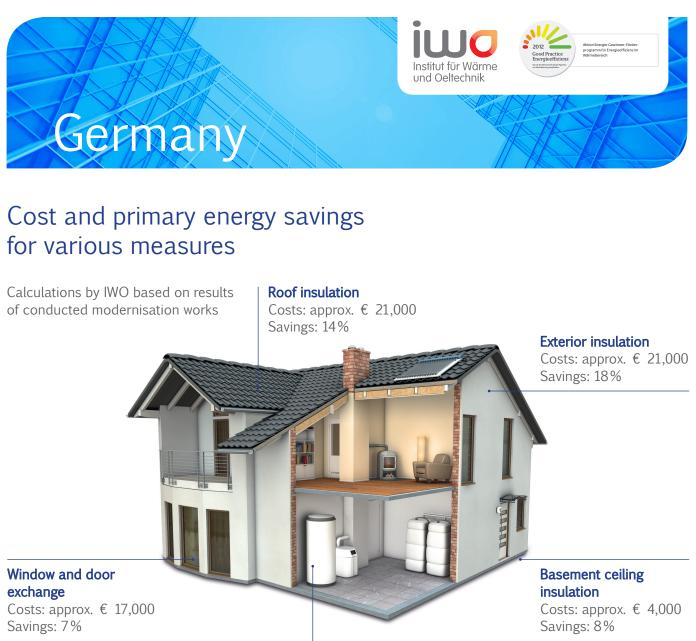
Heating modernisation: Oil condensing boiler with solar Costs: approx. € 22,500 Savings: 38%
